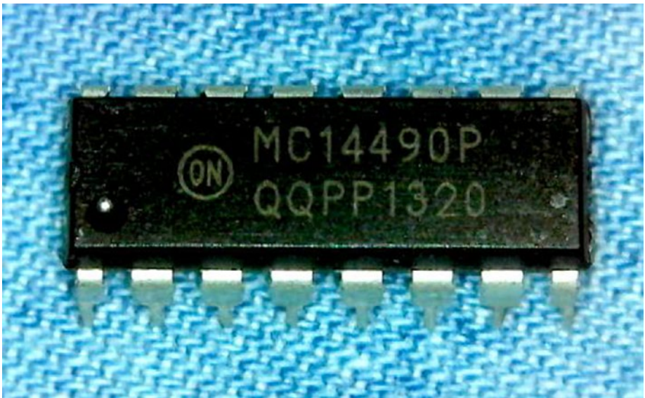
Figure 5-1. The MC14490 dual inline package (DIP) chip
